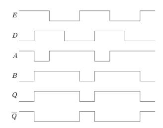
(b) From the timing diagram we see that when E = 1, Q follows D faithfully, while when E = 0, Q does not change. The system is thus a transparant latch.
