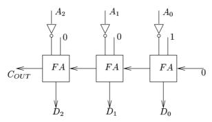
6. Now implement the inverse operation, i.e. one that takes D2, D1, D0 and produces the output (A2,A1,A0). (HINT! Remember how to perform subtraction using 2-complements)
