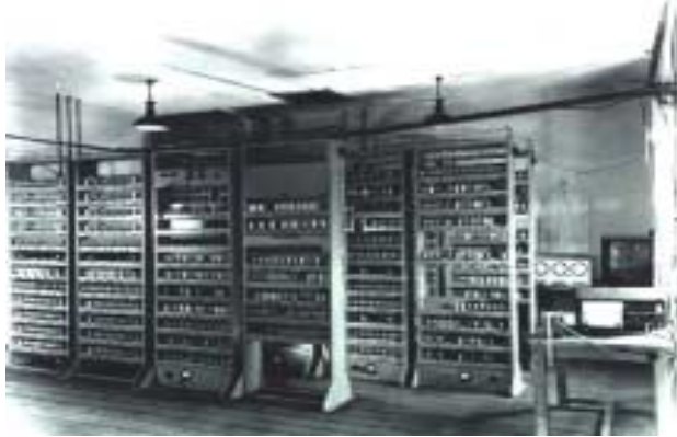
EDSAC, First operational Von Neuman Computer. Pictured 1949
