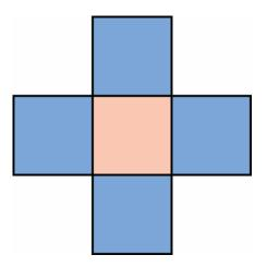
2. This structuring element consists of 5 pixels organized in a cross, let's consider the pink pixel in the center the origin of the structuring element.
