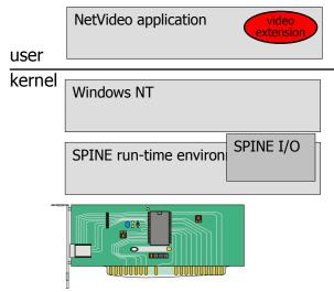
perform video client operations on-board a Myrinet network card (33 Mhz LANai CPU, 256 KB SRAM)
