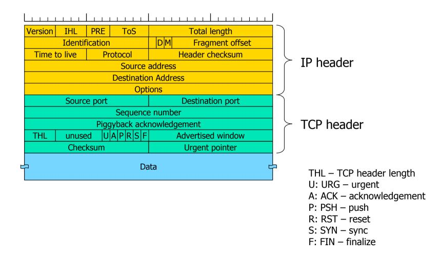
• TCP/IP Header Format for TCP SACK and FACK
