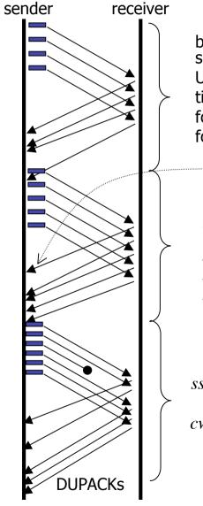
$b_k$  = estimate number of bytes sent in this RTT. Uses average difference of time(sent) and time(ack'd) for every packet for this RTT
