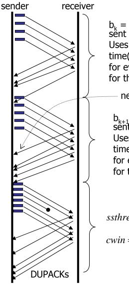
$b_k$  = estimate number of bytes sent in this RTT. Uses average difference of time(sent) and time(ack'd) for every packet for this RTT
