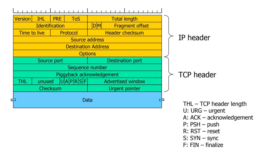
TCP/IP Header Format for TCP SACK and FACK
