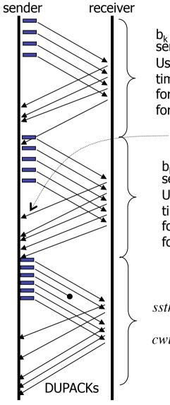
$b_k$  = estimate number of bytes sent in this RTT. Uses average difference of time(sent) and time(ack'd) for every packet for this RTT
