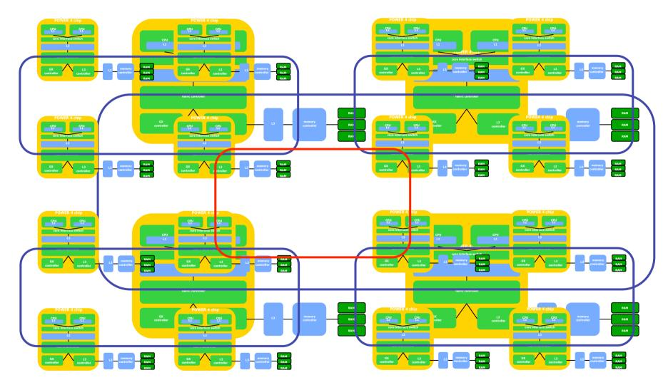
**Chip-chip fabric** in fabric controller can connect 4 multi-chips into a 4x4 chip, 2-way SMP  $\rightarrow$  32-way MP
