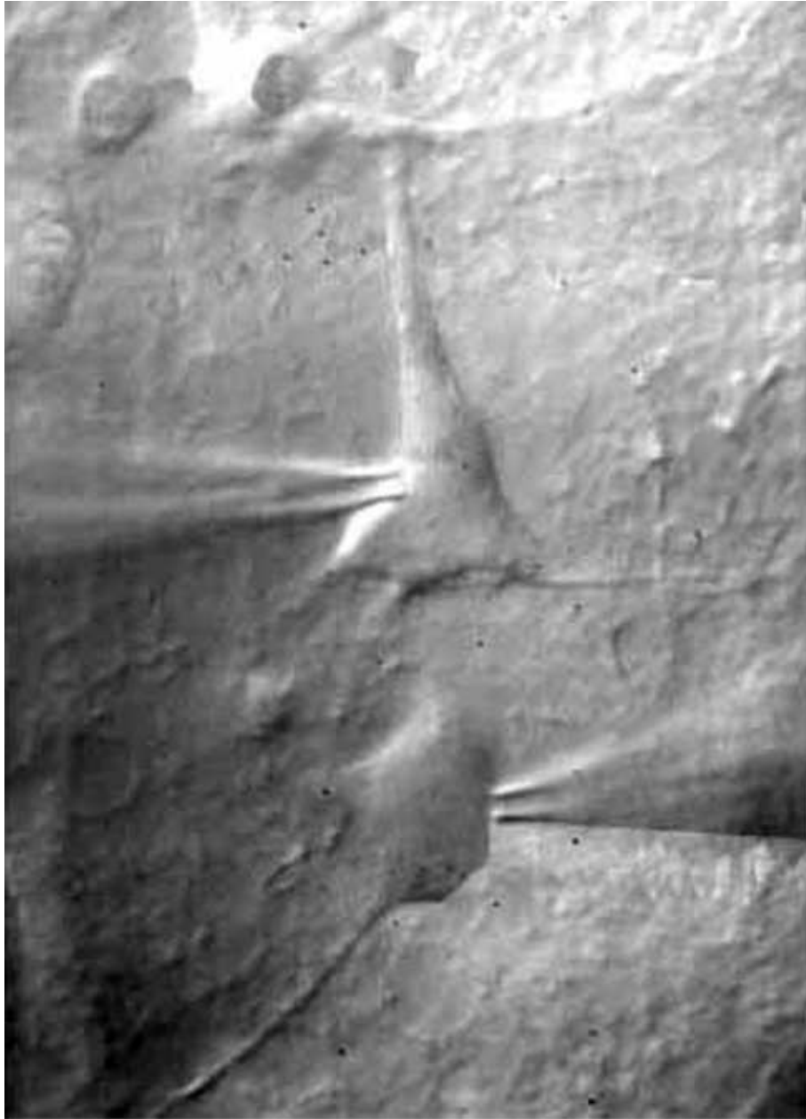
Figure 2.5: Patch clamp electrodes onto two neurons in in vitro preparation under a phase contrast microscope[63]
