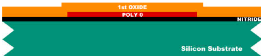
FIGURE 1.5. A 2.0\ \mu\text{m} layer of PSG is deposited on the wafers by low pressure chemical vapor deposition (LPCVD). This is the first sacrificial layer.
