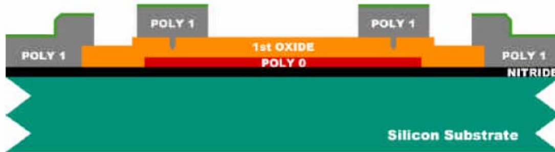
FIGURE 1.9. The wafer is coated with photoresist and the fourth level (POLY1) is lithographically patterned. The PSG is first etched to create a hard mask and then Poly 1 is etched by RIE. After the etch is completed, the photoresist and PSG hard mask are removed.
