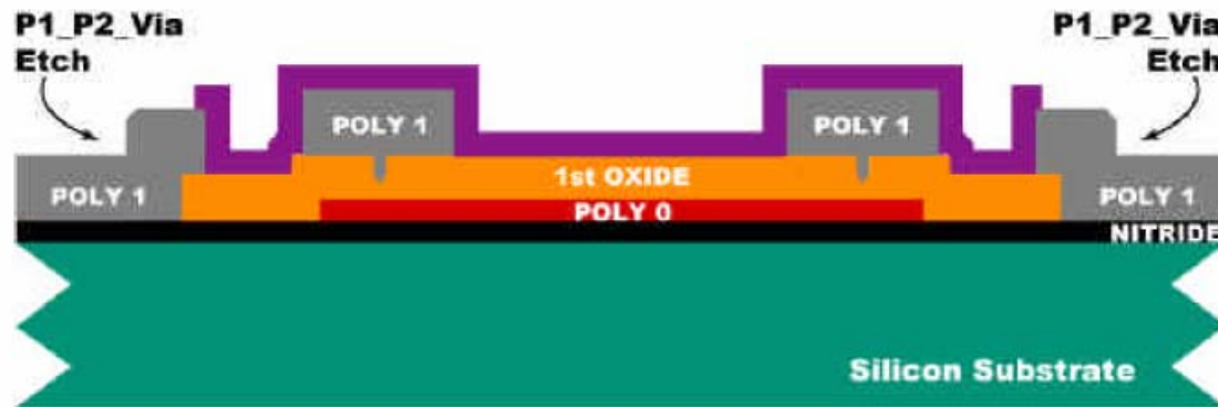
FIGURE 1.11. The wafer is coated with photoresist and the fifth level (POLY1_POLY2_VIA) is lithographically patterned. The unwanted Second Oxide is RIE etched, stopping on Poly 1, and the photoresist is stripped.
