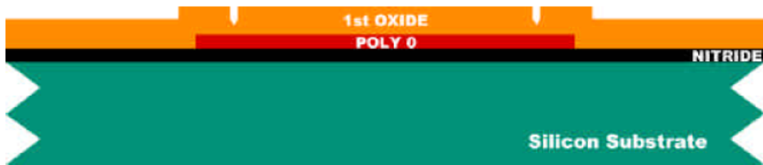
FIGURE 1.6. The wafers are coated with photoresist and the second level (DIMPLE) is lithographically patterned. The dimples, 750 nm deep, are reactive ion etched into the first oxide layer. After the etch, the photoresist is stripped.
