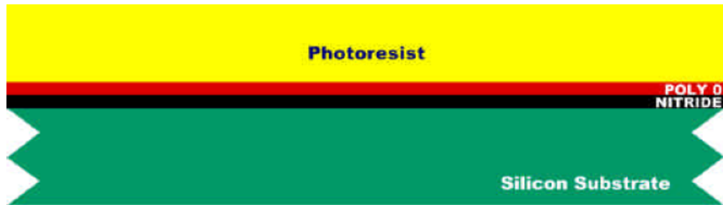
FIGURE 1.2. The surface of the starting n-type (100) wafers are heavily doped with phosphorus in a standard diffusion furnace using \text{POCl}_3 as the dopant source. A 600 nm blanket layer of low stress silicon nitride (Nitride) is deposited followed by a blanket layer of 500 nm polysilicon (Poly 0). The wafers are then coated with UV-sensitive photoresist.
