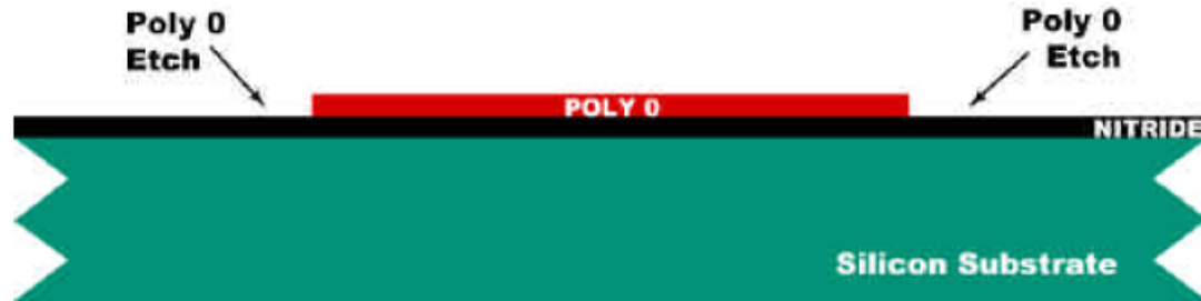
FIGURE 1.4. Reactive ion etching (RIE) is used to remove the unwanted polysilicon. After the etch, the photoresist is chemically stripped in a solvent bath. This method of patterning the wafers with photoresist, etching and stripping the remaining photoresist is used repeatedly in the PolyMUMPs process.
