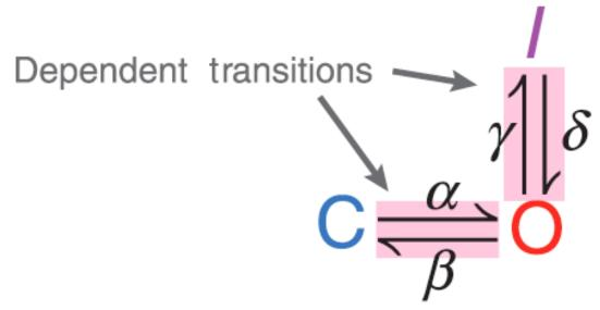
Hypothetical channel; inactivation can only occur from the open state, i.e. state to state transitions are dependent
