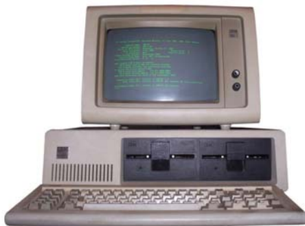
International Business Machines Personal Computer 5150 med Microsoft Disc Operating System (IBM PC med MS-DOS)
