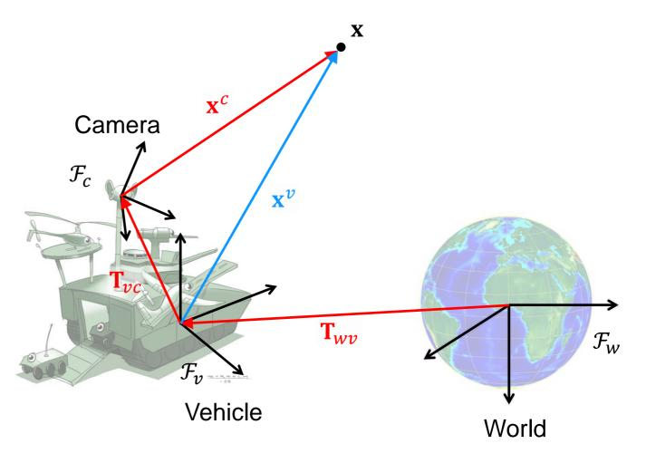
A point x has a known position relative to a camera mounted on a vehicle  $x^c$
