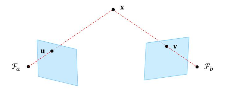
Two perspective cameras observing the same scene point, puts a strong constraint on how the two cameras must be positioned and oriented, both relative to the scene and each other
