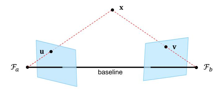
• The **baseline** is the line joining the two camera centers
