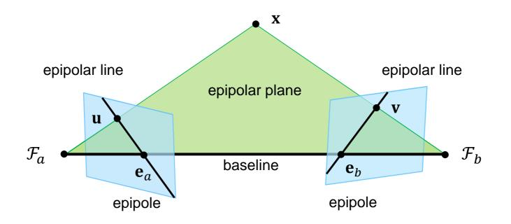
The geometry of two cameras observing the same scene is known as epipolar geometry
