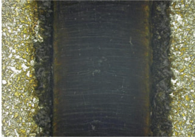
FIGURE 4. High pulse energy fiber laser technology delivered through a novel square fiber efficiently ablates the AISi coating to expose the native HSS surface for enhanced weld quality.
