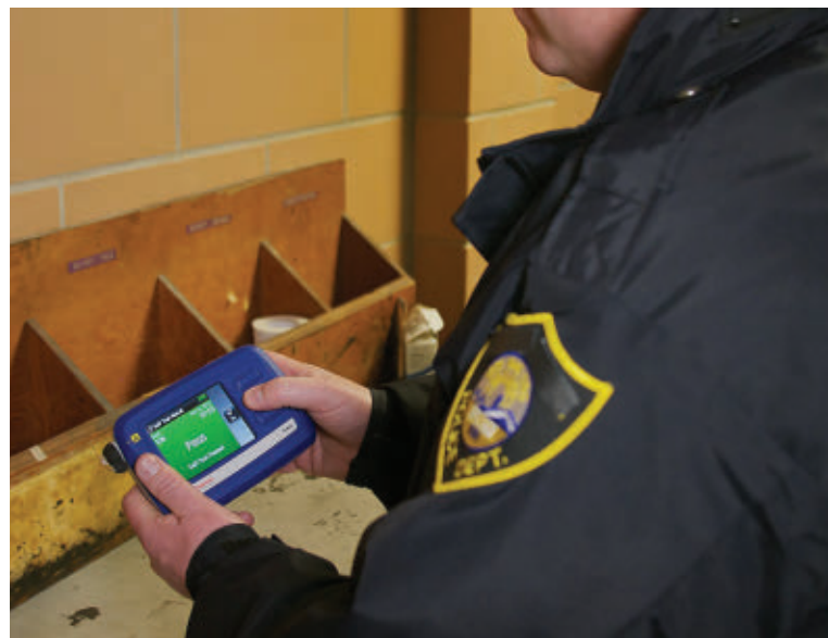
FIGURE 4. The TruNarc Raman spectrometer provides noncontact, nondestructive testing for controlled substances for law enforcement. (Courtesy of Thermo Fisher Scientific)
