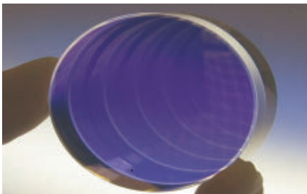
Solid, air spaced and piezo tunable etalons with a total thickness variation of < 3nm
