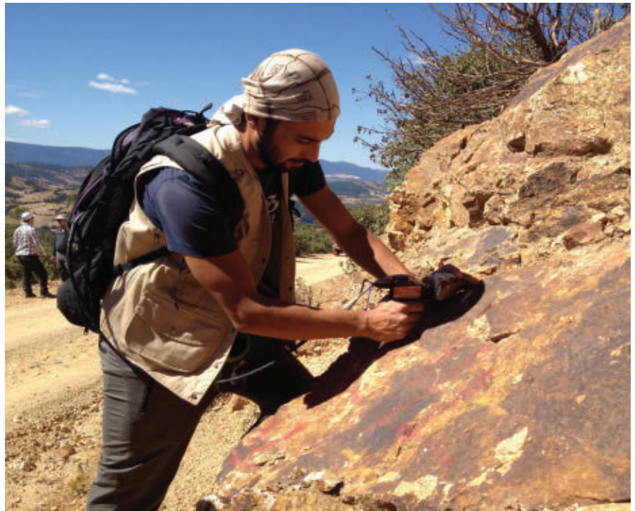
FIGURE 2. The OreXpress spectrometer identifies minerals by comparing spectral traces against a library of 1500 known mineral spectra. (Courtesy of Spectral Evolution)
