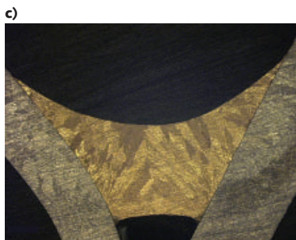
FIGURE 3. A comparison of single-spot (a) and trifocal (b) brazed seams that join steel with CuSi wire. An improved finish and suppression of edge roughness is evident in the trifocal brazing example. A cross-section (c) highlights the joint uniformity and quality obtainable with trifocal brazing.
