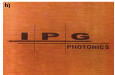
FIGURE 5. Example of the fine, nodular Cu surface structure (10,000X magnification) obtained using a sub-nanosecond NIR fiber laser (a). The textured Cu surface is perfectly black, making it an ideal absorber for subsequent laser processing (b).
