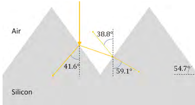
Figure 2.2.5.: Light incident on a pyramidal structure will have at least two chances of transmission into the Si. In combination with an anti-reflection coating this structure may yield a very low front-side reflection.
