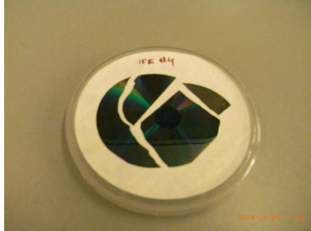
Figure 5.3.5.: A two inch Si wafer with a thickness of 50\ \mu\text{m} is imprinted with a periodic structure using nanoimprint lithography. The wafer broke during demolding.
