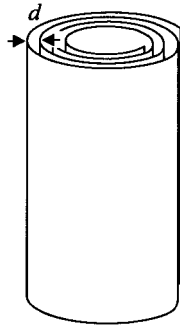
Fig. 7. In model C , a metallic sheet is wound around each cylinder in a coil. Each turn of the coil is spaced by a distance d from the previous sheet.
