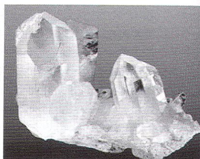
Figure 4-35. Synthetic quartz crystal (left) and rock crystal (right).
