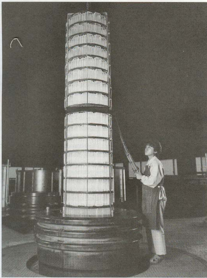
Figure 2.11. Growth of quartz crystals in the world's largest autoclave. (Photo courtesy of Dr. Taki.)
