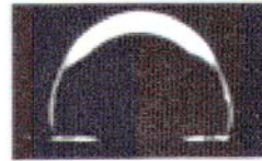
Figure 4-64. Different wetting behavior on a surface: a) the liquid spreads easily over the surface; b) the liquid wets the surface partly; and c) the liquid does not wet the surface. Corresponding to the drawings, a water droplet on a hydrophilic (b) and a hydrophobic surface (c) is shown.
