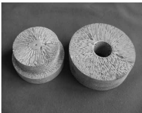
Fig. 4. Magnesium gasar with axial (left) and radial (right) pores.
