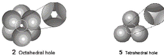
Figure 1-5. Octahedral and tetrahedral hole in close-packed layers of spheres. From Shriver and Atkins; Inorganic Chemistry .
