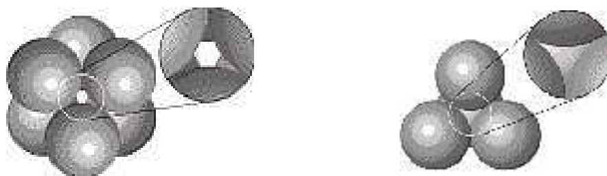
Figure 1-8. Octahedral (left) and tetrahedral (right) void in close-packed layers of spheres.
