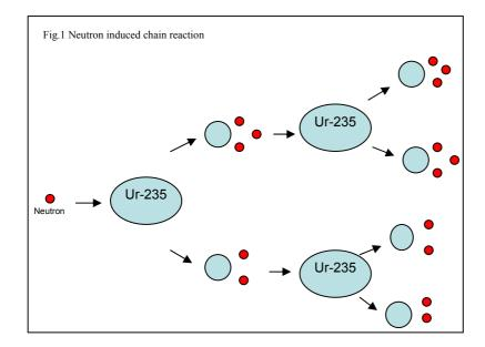
If the numbers of neutrons are just sufficient to keep the reaction in balance, the result is a 'critical reactor' – and a self-sustained chain reaction is achieved. U-235 and Pu-239 nuclides capture a neutron and thereby we get a fission, producing 200 MeV of heat pr neutron. The heat is used to make steam, which drives electricity-producing turbines.
