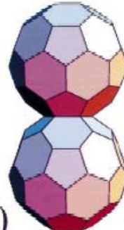
Fig. 2. The structures of two cubic Fibonacci approximants with Bergman clusters (BC) shown as solid soccer balls: (a) b.c.c. packing of BC in the crystal structure of 1/1-(\text{Al,Zn})_3\text{Mg}_2 ; the connection of Bergman clusters as found in the 1/1 - and 2/1 -approximant: (b) clusters along twofold axes are connected via common edges (b bonds) and (c) along threefold axes via common hexagon faces (c bonds); (d) the rhombohedral packing of BCs at the vertices of prolate and oblate rhombohedra in the crystal structure of 2/1-(\text{Al,Zn})_{3+8}\text{Mg}_{2-8} .
