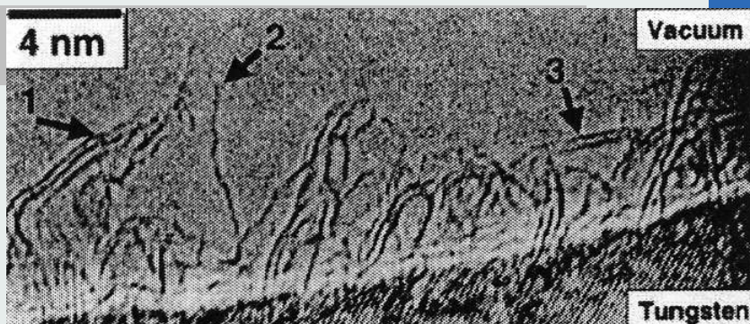
Fig. 36 HREM image of single-walled BN nanotubes adhering on a W substrate. (Reproduced with permission from ref. 110).
