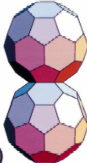
Fig. 2. The structures of two cubic Fibonacci approximants with Bergman clusters (BC) shown as solid soccer balls: (a) b.c.c. packing of BC in the crystal structure of 1/1-(Al,Zn)_3Mg_2 ; the connection of Bergman clusters as found in the 1/1 - and 2/1 -approximant: (b) clusters along twofold axes are connected via common edges (b bonds) and (c) along threefold axes via common hexagon faces (c bonds); (d) the rhombohedral packing of BCs at the vertices of prolate and oblate rhombohedra in the crystal structure of 2/1-(Al,Zn)_{3+g}Mg_{2-g} .
