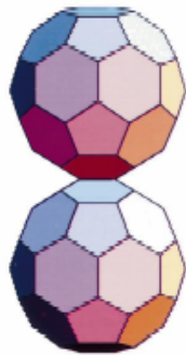
Fig. 2. The structures of two cubic Fibonacci approximants with Bergman clusters (BC) shown as solid soccer balls: (a) b.c.c. packing of BC in the crystal structure of 1/1-(Al,Zn)_3Mg_2 ; the connection of Bergman clusters as found in the 1/1 - and 2/1 -approximant: (b) clusters along twofold axes are connected via common edges (b bonds) and (c) along threefold axes via common hexagon faces (c bonds); (d) the rhombohedral packing of BCs at the vertices of prolate and oblate rhombohedra in the crystal structure of 2/1-(Al,Zn)_{3+g}Mg_{2-g} .
