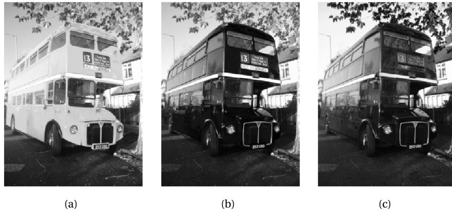
Figure 8.5. The red (a), green (b), and blue (c) components of the colour image in figure 8.1.
