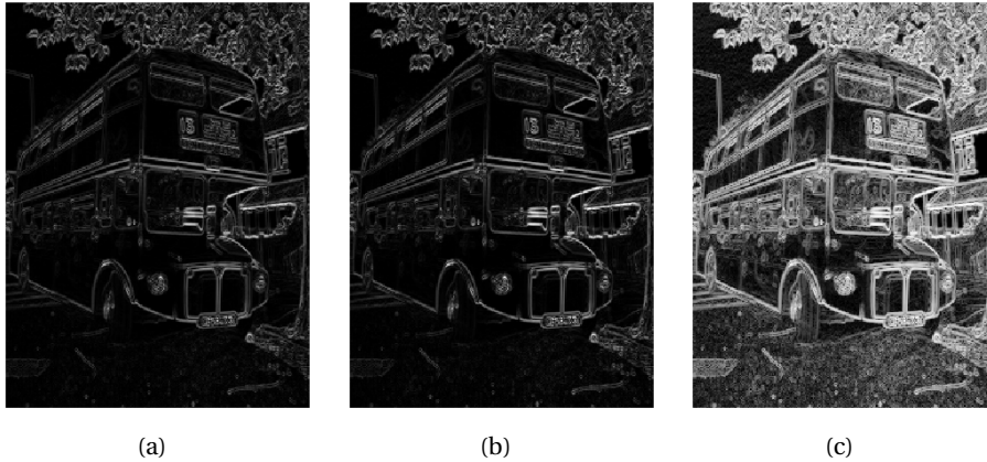
Figure 8.11. Computing the gradient. The image obtained from the computed gradient is shown in (a) and in (b) the numbers have been normalised. In (c) the contrast has been enhanced with a logarithmic function.
