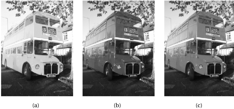
Figure 8.6. Alternative ways to convert the colour image in figure 8.1 to a grey level image. In (a) each colour triple has been replaced by its maximum, in (b) each colour triple has been replaced by its sum and the result mapped to [0, 1] , while in (c) each triple has been replaced by its length and the result mapped to [0, 1] .
