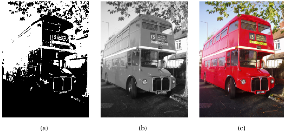
Figure 16.1. Different version of the same image; black and white (a), grey-level (b), and colour (c).
