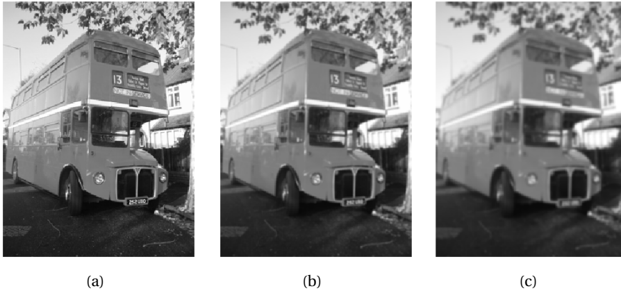
Figure 16.9. The images in (b) and (c) show the effect of smoothing the image in (a).
