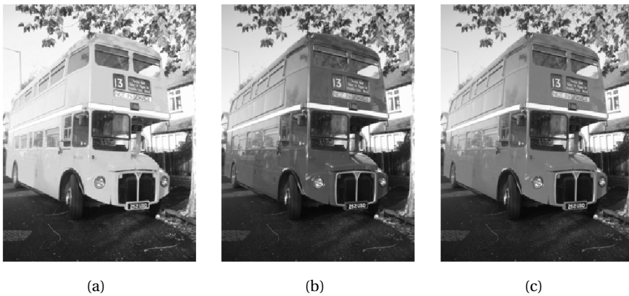
Figure 15.6. Alternative ways to convert the colour image in figure 15.1 to a grey level image. In (a) each colour triple has been replaced by its maximum, in (b) each colour triple has been replaced by its sum and the result mapped to [0, 1] , while in (c) each triple has been replaced by its length and the result mapped to [0, 1] .
