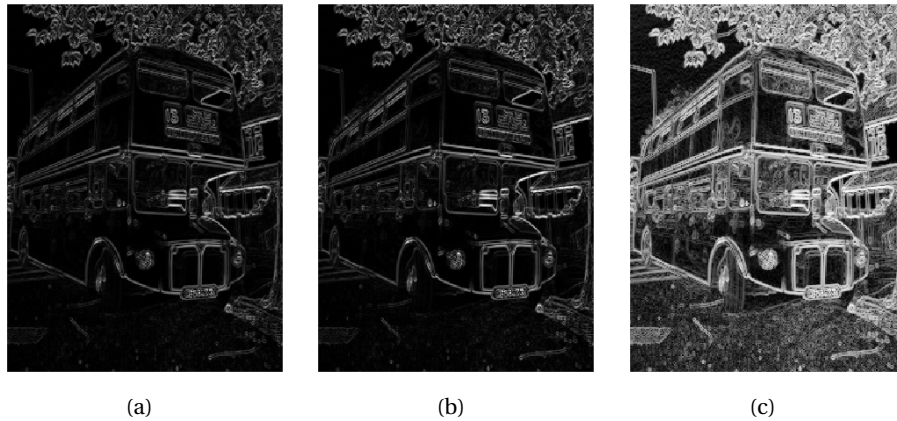
Figure 15.11. Computing the gradient. The image obtained from the computed gradient is shown in (a) and in (b) the numbers have been normalised. In (c) the contrast has been enhanced with a logarithmic function.
