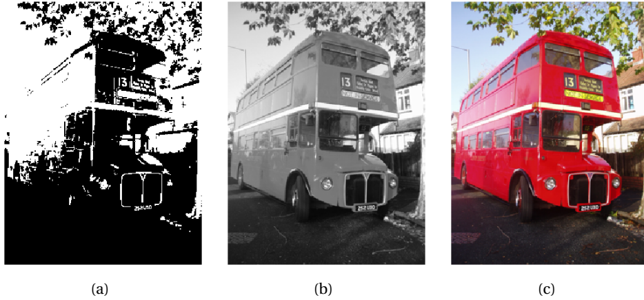
Figure 15.1. Different version of the same image; black and white (a), grey-level (b), and colour (c).
