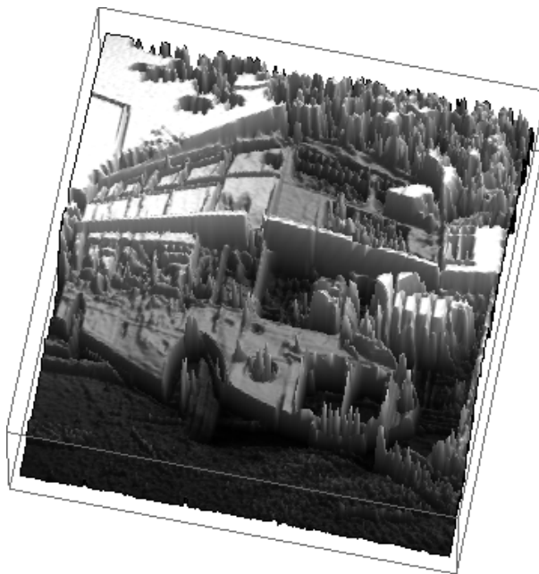
Figure 15.3. The grey-level image in figure 15.1 plotted as a surface. The height above the (x, y) -plane is given by the intensity value.
