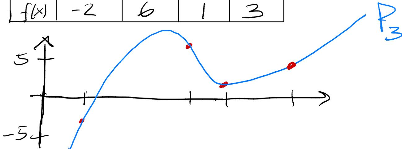
Newtonform:  $P_3(x) = c_0 + c_1(x+5) + c_2(x+5)(x+1) + c_3(x+5)(x+1)x$
