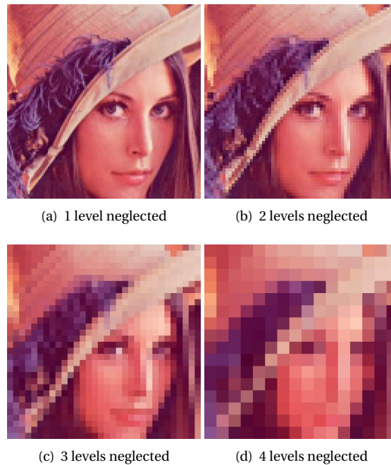
Figure 10.9: Image of Lena, with higher levels of detail neglected for the Haar wavelet.
