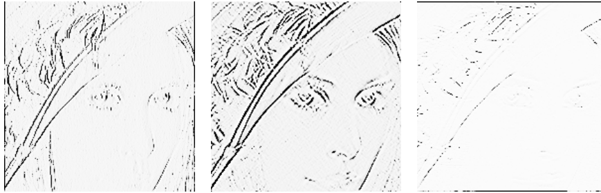
(a) The second-order partial derivatives in the x -direction (b) The second-order partial derivatives in the xy -direction (c) The second-order partial derivatives in the y -direction
