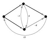
The solution is not optimal, e.g.  $z_{pw} = -8 < 0$ . We now choose to take this variable into the basis. So this edge is going into the tree.
