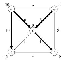
Consider the minimum cost network flow problem based on the directed graph depicted in the figure. The number associated with a directed edge (i, j) is its cost  $c_{ij}$  (per unit flow), and the number associated with a node i is its supply  $b_i$  (negative values represent demands).
