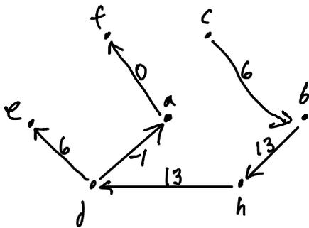
b) Dual variables  $y_j - y_i = C_{ij}$  for  $(i,j)$  in the spanning tree.
