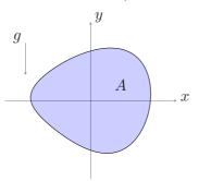
A viscous flow in a duct of arbitrary cross-section (see figure) is driven by a pressure change along the duct. The cross section is parallel to the xy plane and is denoted by A, while the z axis is aligned along the duct. The fluid is incompressible, the dynamic viscosity coefficient is  $\mu$ , gravity is directed in the negative y direction and the duct wall is impenetrable. Moreover, we assume that the flow is stationary and uniform in the z direction.
