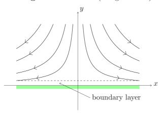
An inviscid solution for stagnation flow at a wall (see figure) is
