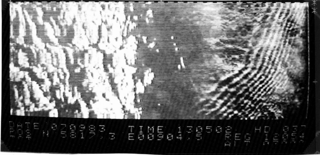
Figure 6.6: Radar echo from the sea surface in an area 10–15 km from shore south-east of Ryvingen between Grimstad and Arendal. The picture was taken on the 7th of September 1983 by a plane used for surveillance of oil pollution. The band structure suggests internal waves with wavelengths from 0.5 to 1 km. Further discussion is found in a paper by Gjevik and Høst (1984). (Photo Fjellanger Widerøe A/S).
