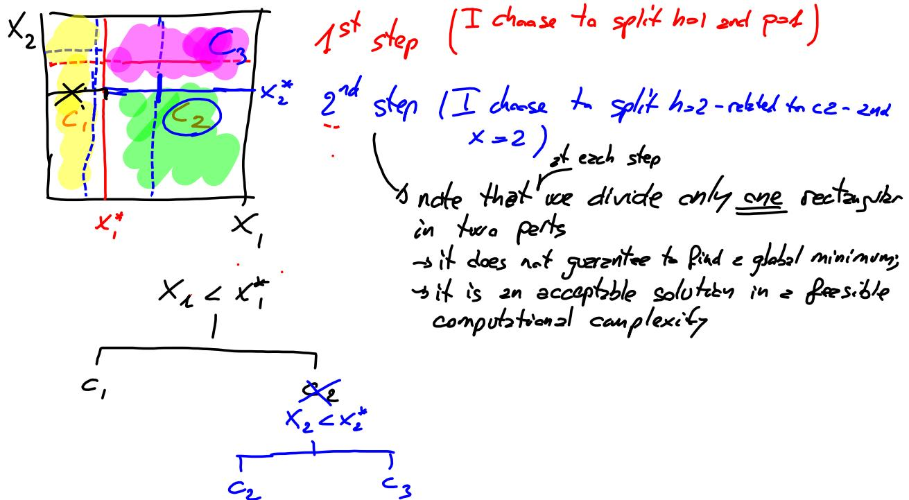
The procedure will lead to a continuous decrease of the variance until each leaf contains only one observation (which corresponds to interpolate)
