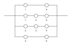
The minimal path sets of a bridge systems are:
