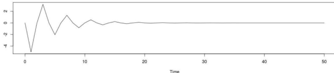
Dynamical system  $\alpha_t = -1.1\alpha_{t-2}$ ,  $t = 2, 3, \dots$ ,  $\alpha_0 = 0, \alpha_1 = -5$
