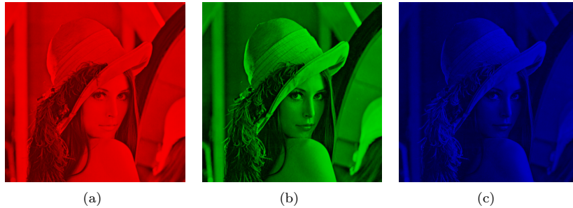
Figure 10.4: The red (a), green (b), and blue (c) components of the colour image in Figure 10.1.
