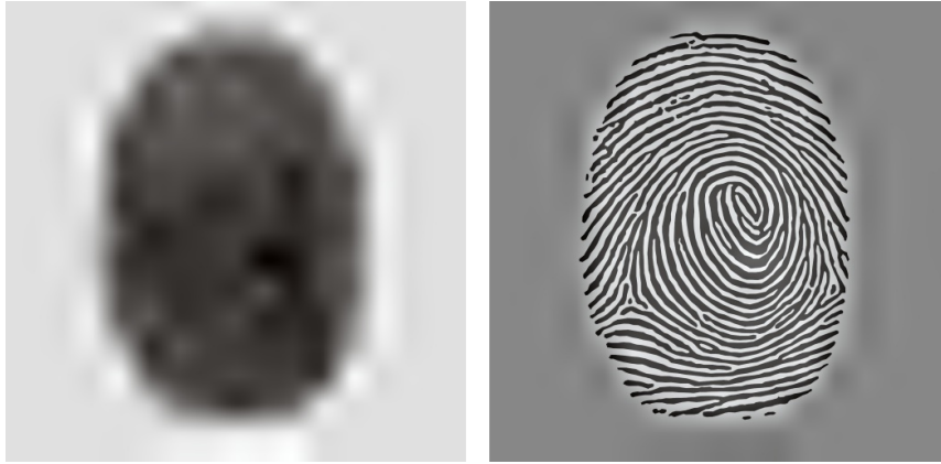
Figure 10.23: The low-resolution approximation and the detail obtained by the FBI standard for compression of fingerprint images, when applied to our sample fingerprint image.
