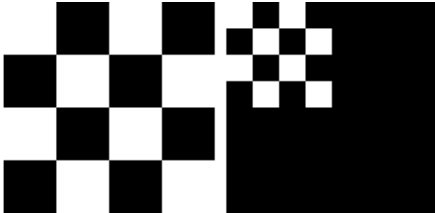
Figure 10.17: A simple image before and after one level of the DWT2. The Haar wavelet was used.
