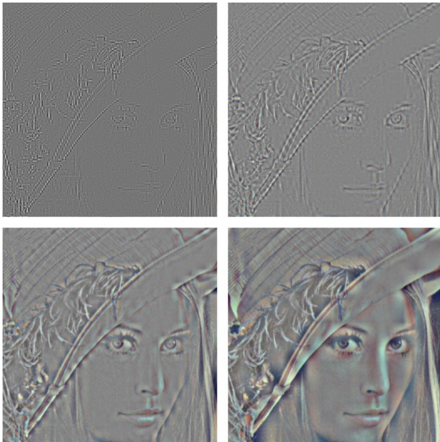
Figure 10.16: The corresponding detail for the image of Lena. The Spline 5/3 wavelet was used.
