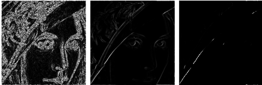
Figure 9.15: The computed gradient (left). In the middle the intensities have been normalised to the [0, 255] , and to the right the contrast has been increased.
