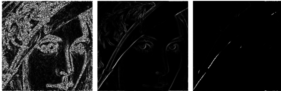
Figure 9.15: The computed gradient (left). In the middle the intensities have been normalised to the [0, 255] , and to the right the contrast has been increased.
