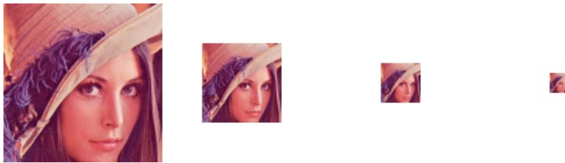
Figure 10.7: The corresponding thumbnail images for the Image of Lena, obtained with a DWT of 1, 2, 3, and 4 levels.
