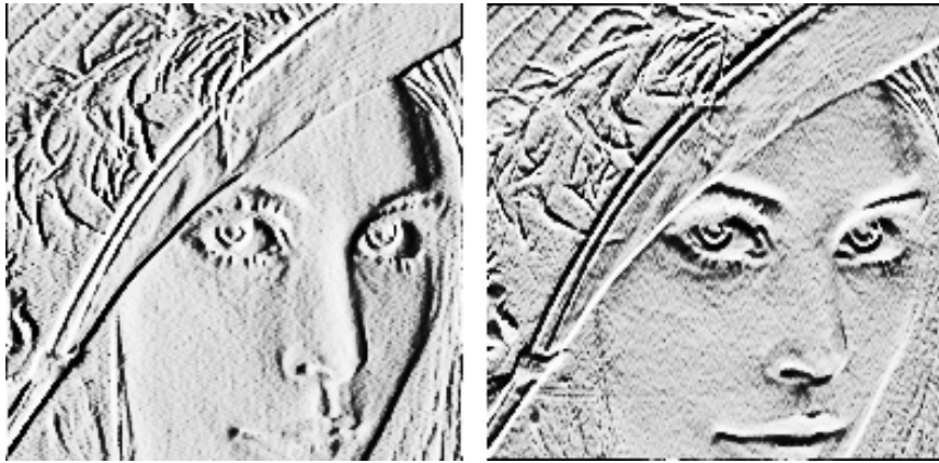
Figure 9.14: The first-order partial derivatives in the x - and y -direction, respectively. In both images, the computed numbers have been normalised and the contrast enhanced.
