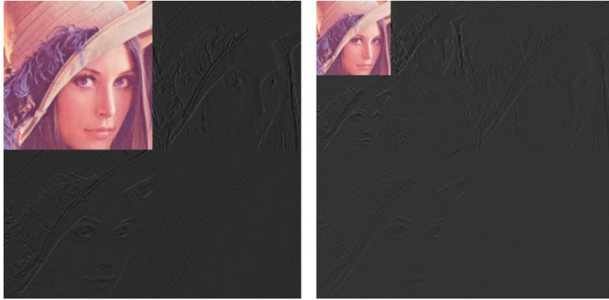
Figure 10.8: The corresponding image resulting from a wavelet transform with the Haar-wavelet for m = 1 and m = 2 .
