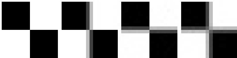
Figure: The results of smoothing the simple image to the left with the filter \frac{1}{4}\{1, \underline{2}, 1\} horizontally, vertically, and both, respectively.
