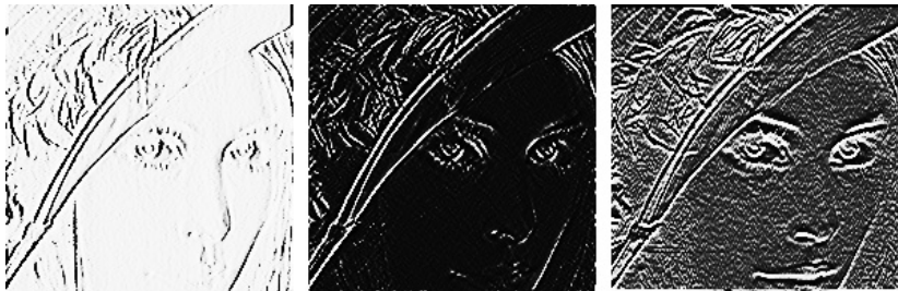
Figure: The second-order partial derivatives in the xx -, xy -, and yy -directions, respectively. In all images, the computed numbers have been normalised and the contrast enhanced.
