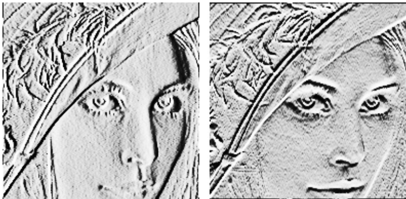
Figure: The first-order partial derivatives in the x - and y -direction, respectively. In both images, the computed numbers have been normalised and the contrast enhanced.
