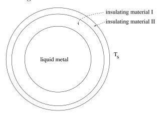
The metal fills the space  $0 \le r \le a$ , while the insulating materials I and II fill the spaces  $a < r \le b$  and  $b < r \le c$ , respectively. A time varying pressure gradient drives the metal flow. Outside the pipe the air temperature is  $T_s$ , and this may vary with time, but not in the space direction along the pipe. In a project we want to calculate how the temperature in the insulating materials vary in time and space.
