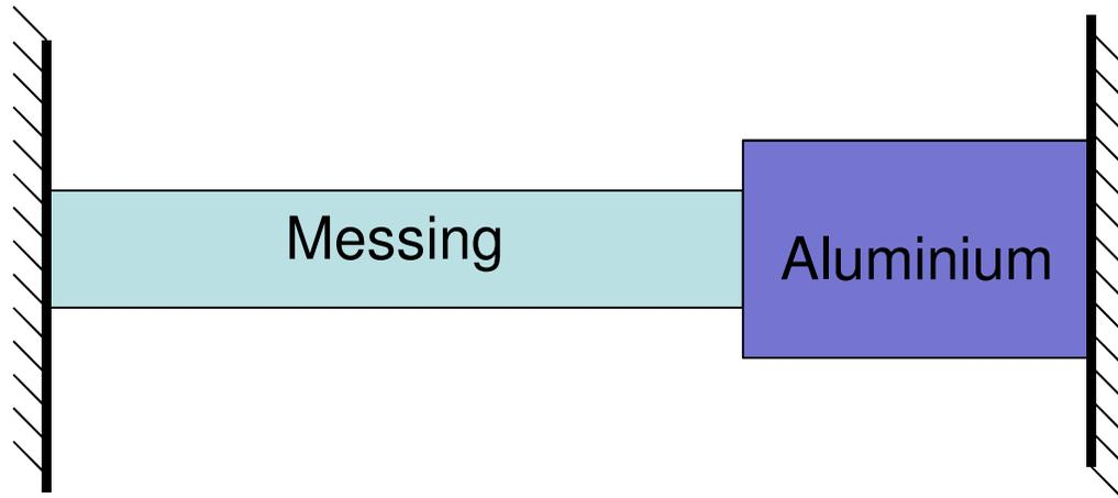
$$\begin{aligned}\epsilon_M &= \frac{\Delta T(-3\alpha_A E_A + 2\alpha_M E_M)}{2(3E_A + E_M)} \\ &= \frac{-20(-3 \times 25 \times 70 + 2 \times 20 \times 90)}{2(3 \times 70 + 90)} \times 10^{-6} = \frac{11}{200000}\end{aligned}$$
